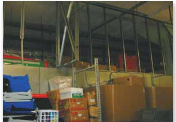
Despite a wire fence, dangerous, heavy items are stored on top of a walk-in cooler—a practice strictly prohibited under federal safety regulations.
